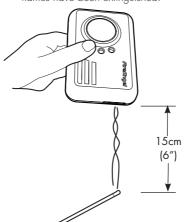
NOTE: If the localised carbon monoxide level within the sensor does not reach 50ppm during the test, the sensor test will stop automatically after 3 minutes.
